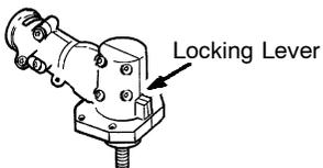
7. Continue to hold in locking lever. This will keep the shaft from turning while tightening the trimmer head.
