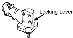
9. Continue to hold in locking lever. This will keep the shaft from turning while tightening the blade nut.
