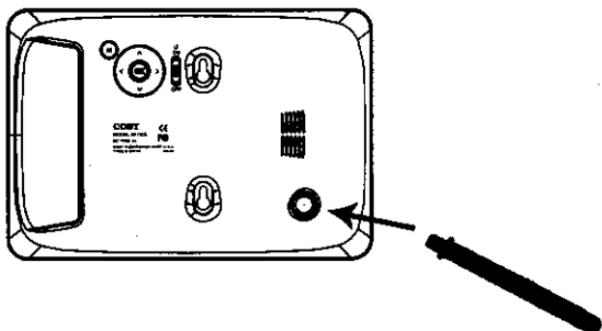
1. Attach the kickstand to the mounting hole.
