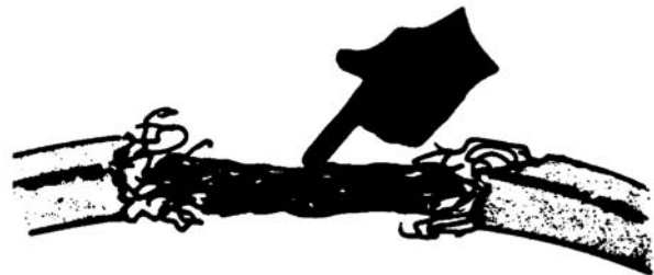
Figure 4-4. Belt Damage Due to Shock Load
