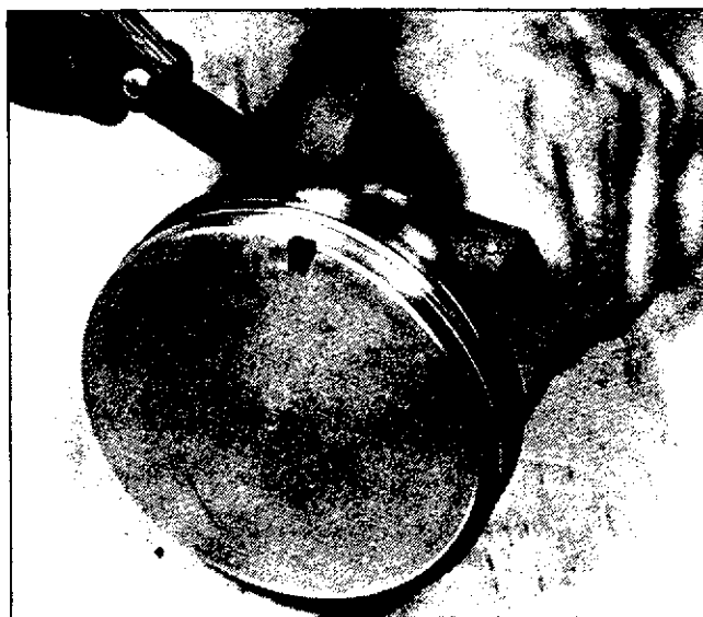
Figure 7-11. Checking Ring Side Clearance
