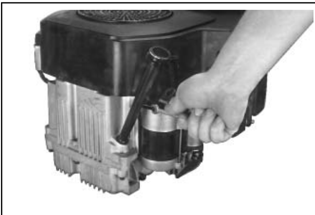
Figure 9-3. Removing Oil Fill Tube Bracket.
