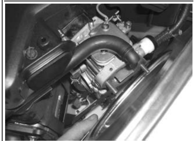
Figure 9-9. Disconnect Breather Hose from Base.
