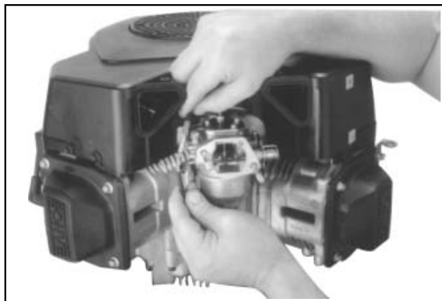
Figure 11-69. Installing External Governor Controls.
