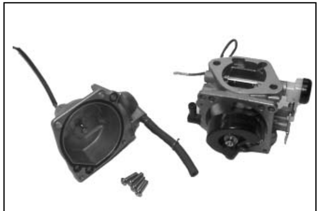
Figure 5-14. Fuel Bowl Removed from Carburetor.
