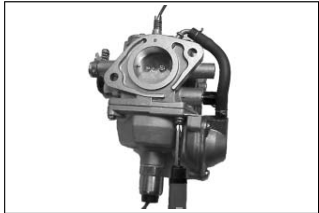
Figure 5-13. Installing Fuel Bowl.
