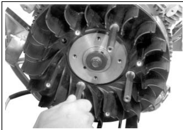
Figure 11-28. Installing Supports for Metal Grass Screen.
