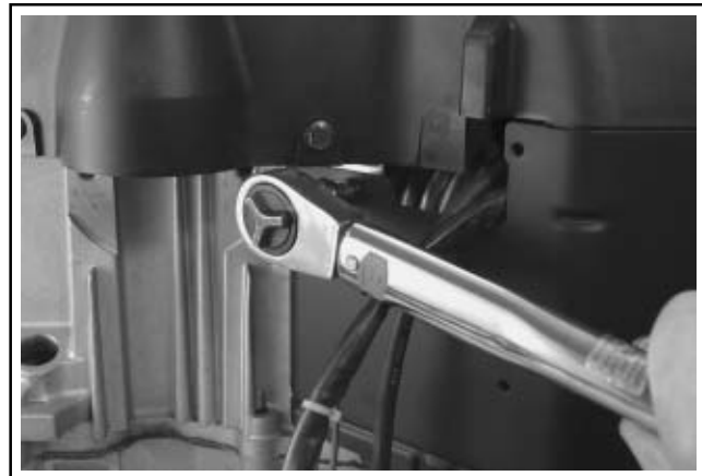
Figure 11-61. Tightening Short Screws for Outer Baffles.
