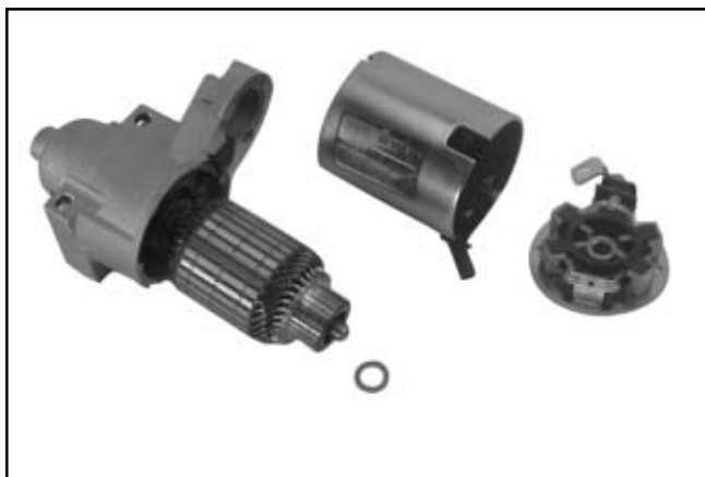
Figure 8-46. Starter Frame Removed.
