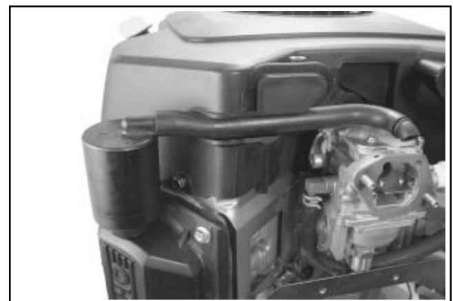
Figure 11-80. Breather Hose and Separator Details.
