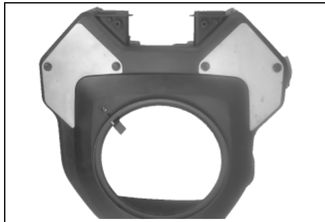
Figure 4-11. Cleanout Kit Installed on Blower Housing.
