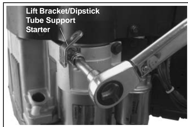
Figure 11-75. Installing Starter and Lift Bracket.
