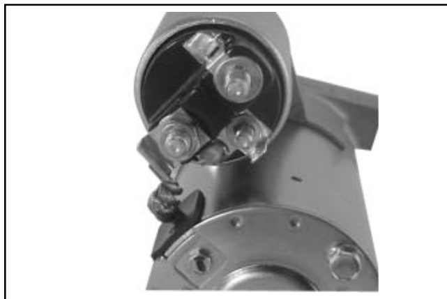
Figure 8-69. Positive (+) Brush Lead Connection.
