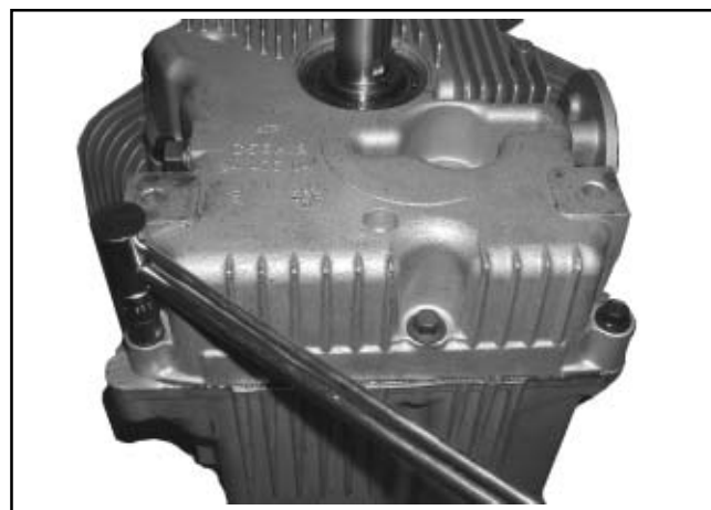
Figure 11-19. Torquing Oil Pan Fasteners.
