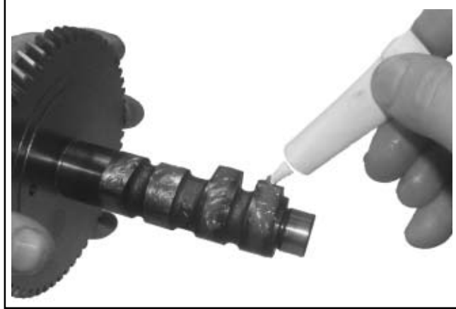
Figure 11-12. Apply Camshaft Lubricant to Cam Lobes.
