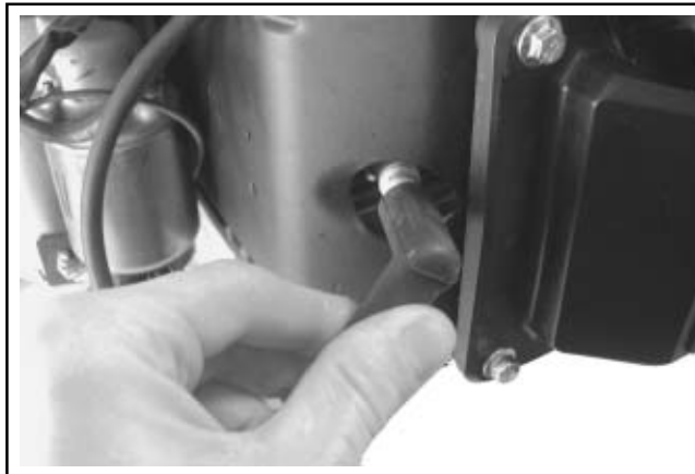
Figure 11-85. Connect Spark Plug Leads.
