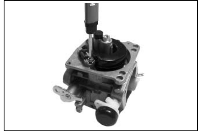
Figure 5-21. Installing Float Assembly.
