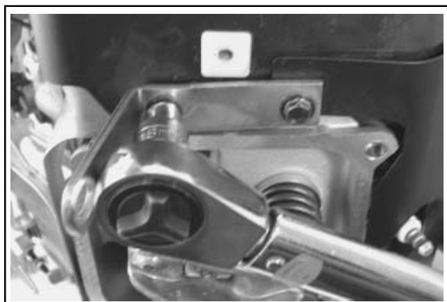
Figure 11-60. Tightening Outer Baffle Front Screws.
