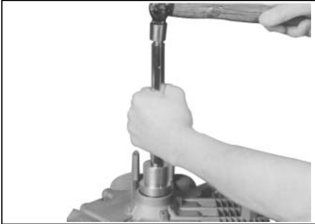
Figure 11-2. Installing Oil Seal in Crankcase.
