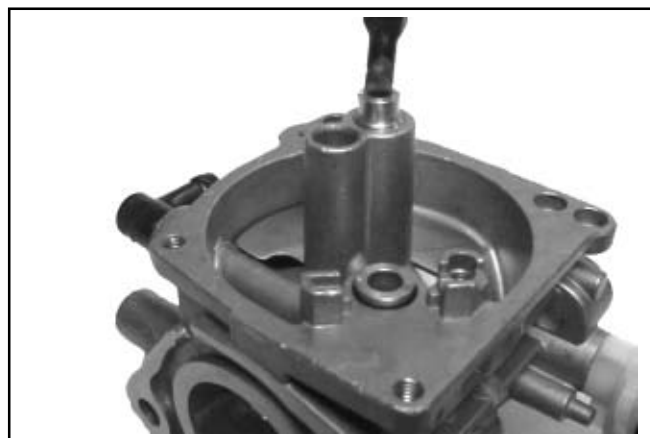
Figure 5-17. Installing Main Nozzle and Main Jet.
