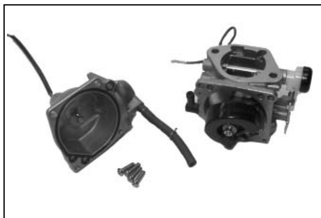
Figure 5-8. Fuel Bowl Removed from Carburetor.
