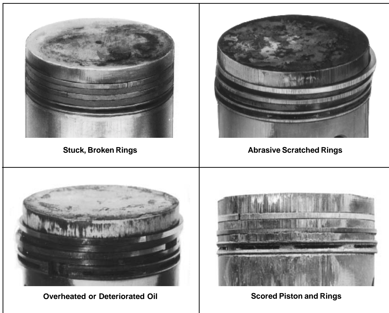
Figure 10-8. Common Types of Piston Damage.
