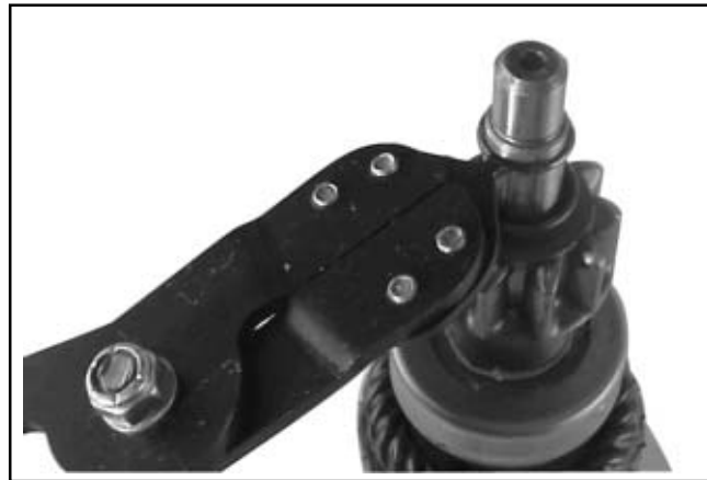
Figure 8-50. Removing Retaining Ring.
