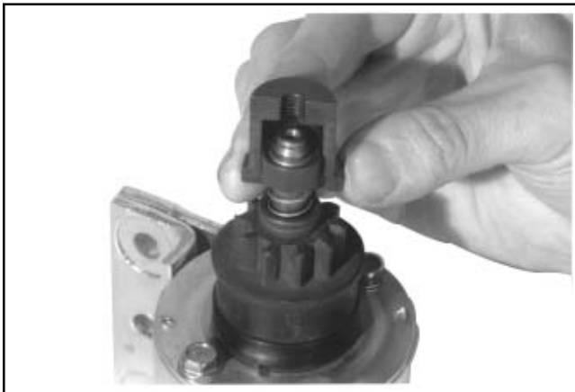
Figure 8-34. Assembling Larger Inner Half Around Spring Retainer.
