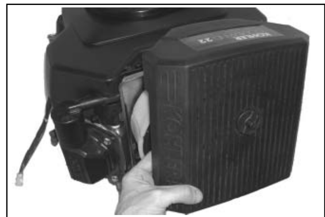
Figure 9-5. Removing Standard Air Cleaner Cover.
