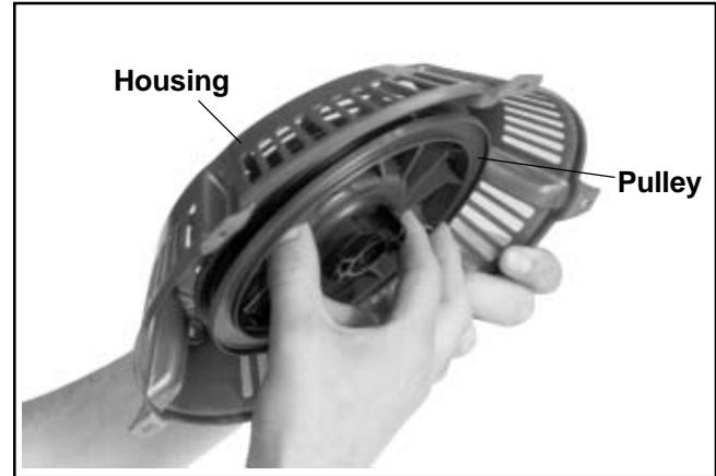
Figure 7-6. Removing Pulley from Housing.
