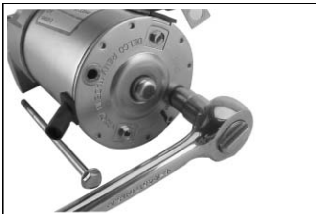
Figure 8-44. Removing Thru Bolts.
