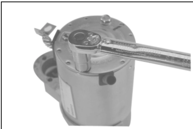
Figure 8-67. Torquing Thru Bolts.
