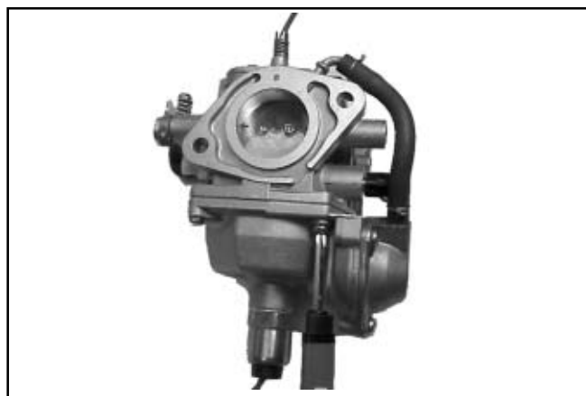
Figure 5-24. Installing Fuel Bowl.
