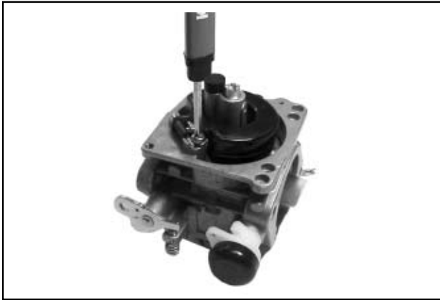
Figure 5-11. Installing Float Assembly.
