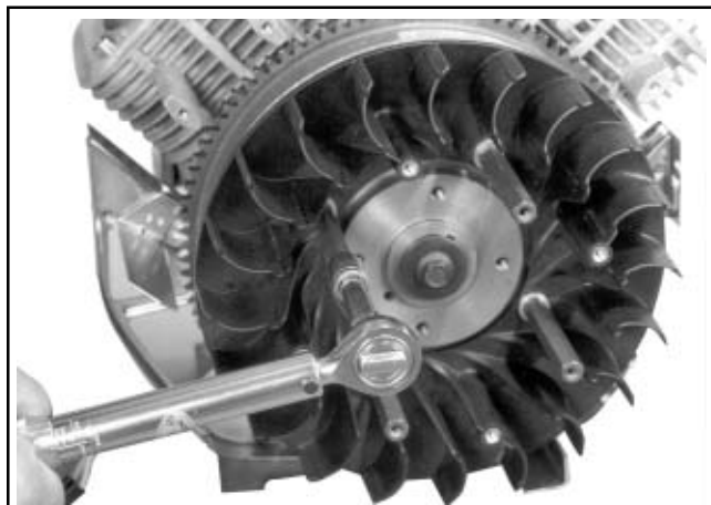
Figure 11-29. Torquing Supports for Metal Screen (Some Models).
