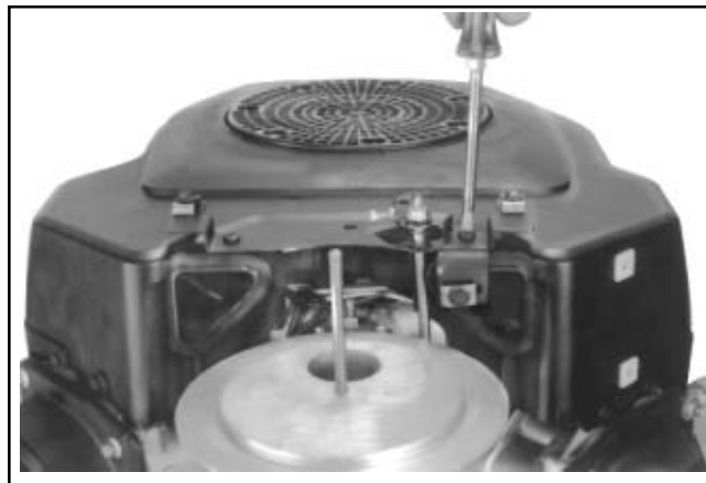
Figure 11-71. Installing Control Panel.
