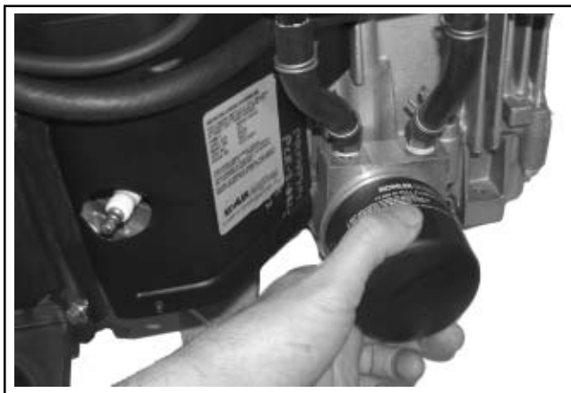
Figure 9-4. Removing Oil Filter.
