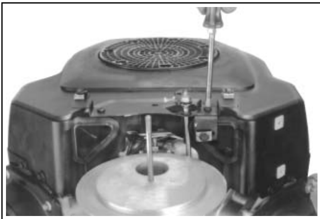
Figure 9-11. Removing Control Panel.
