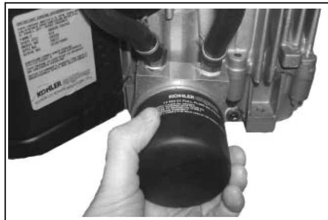
Figure 11-83. Installing and Tightening Oil Filter.
