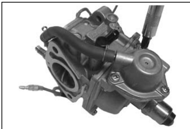
Figure 5-31. Installing Accelerator Pump Housing Screws and Hose.
