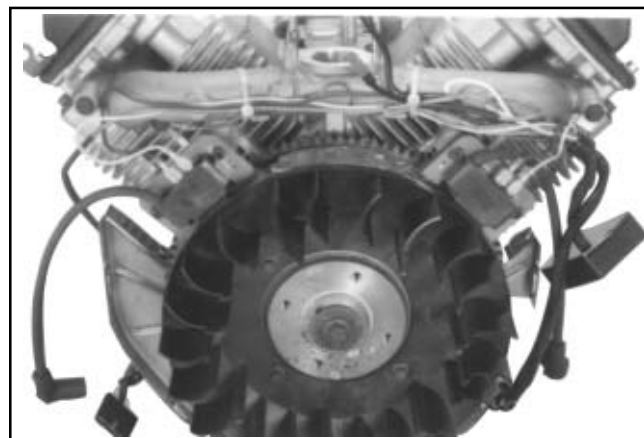
Figure 9-33. Position of Ignition Modules.
