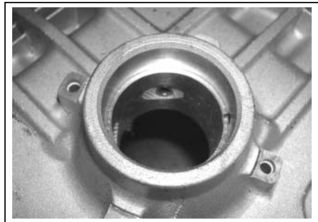
Figure 11-1. Seal Bore of Crankcase.
