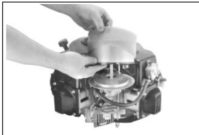
Figure 9-8. Removing Commercial Mower Element and Precleaner.
