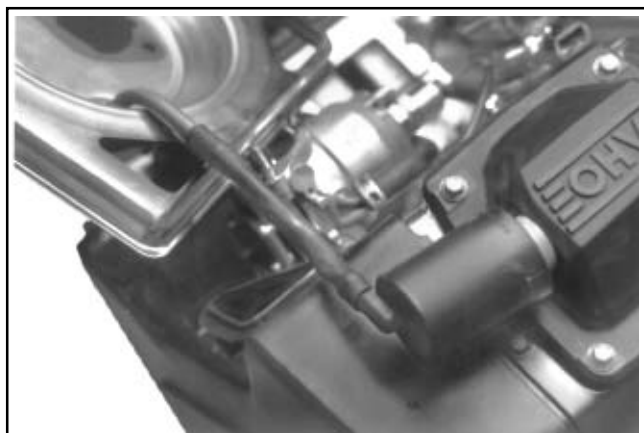
Figure 9-8. Removing Commercial Mower Element and Precleaner.
