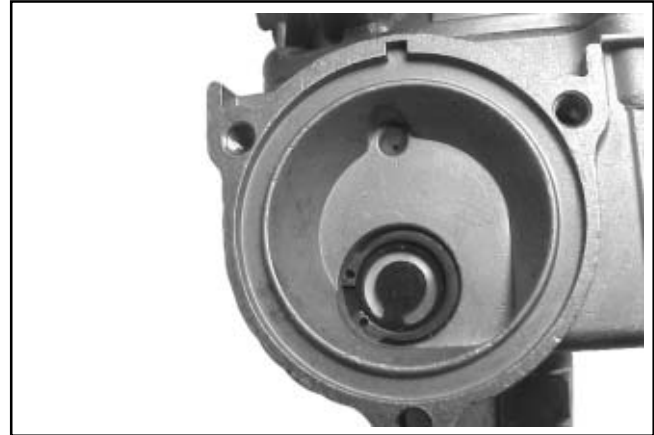
Figure 5-29. Check Valve and Retaining Ring Installed.
