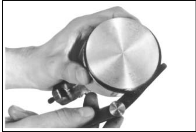
Figure 10-10. Measuring Piston Ring Side Clearance.
