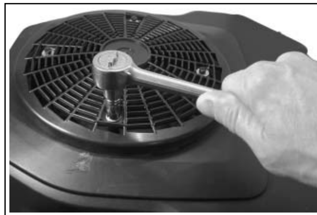
Figure 9-24. Removing Flywheel Screen.
