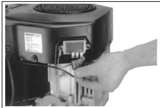
Figure 11-65. Attaching Connector Plug.
