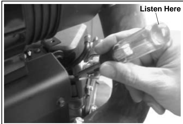
Figure 5B-17. Checking Injectors.
