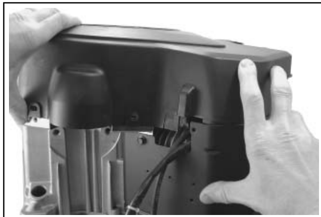
Figure 11-59. Installing Blower Housing.
