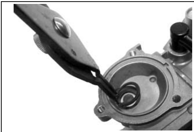
Figure 5-28. Removing Retaining Ring.
