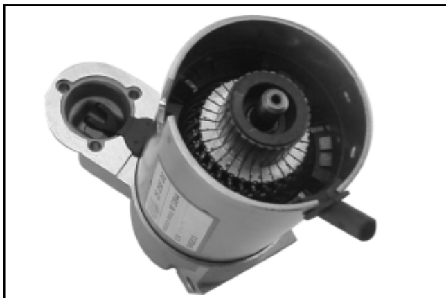
Figure 8-58. Installing Frame and Drain Tube.
