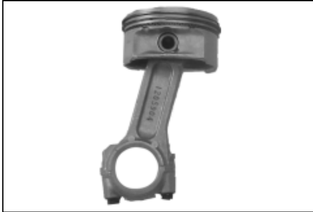
Figure 11-6. Connecting Rod Configuration to Piston with the Part Number "up".
