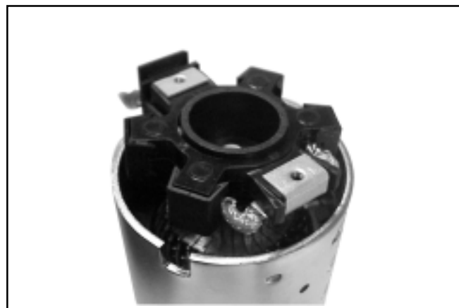
Figure 8-60. Installing Brush Holder Assembly With Supplied Tube.
