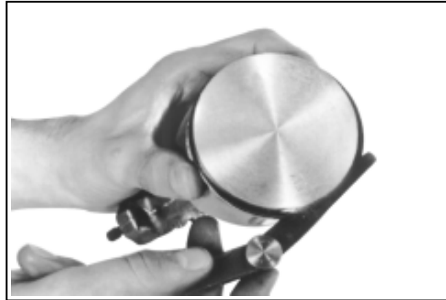
Figure 10-9. Measuring Piston Ring Side Clearance.
