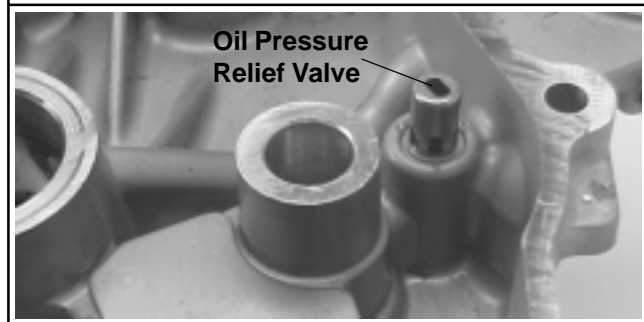
Figure 6-8. Oil Pressure Relief Valve Styles.
