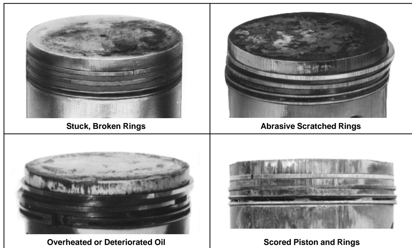
Figure 10-7. Common Types of Piston and Ring Damage.
