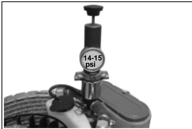
Figure 7-13. Adapter and Tester Installed.
