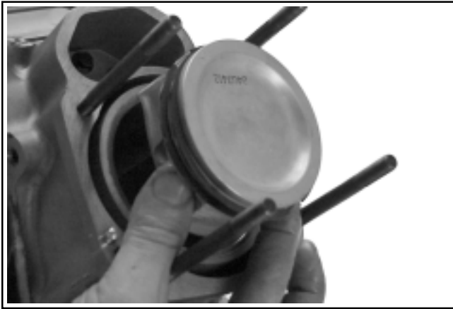
Figure 9-78. Removing Connecting Rod and Piston Assembly.
