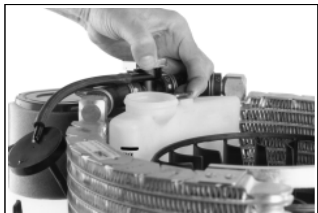
Figure 7-7. Tipping Bracket Away after Removing Reservoir Cap.
