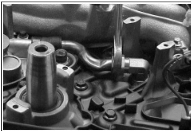
Figure 9-44. Removing Hex. Cap Section.
