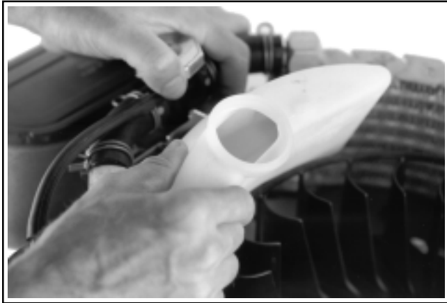
Figure 7-8. Removing Overflow Reservoir.
