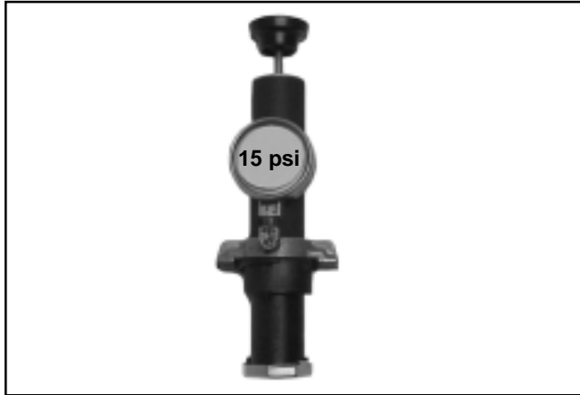
Figure 7-12. Adapter Installed onto the Tester.
