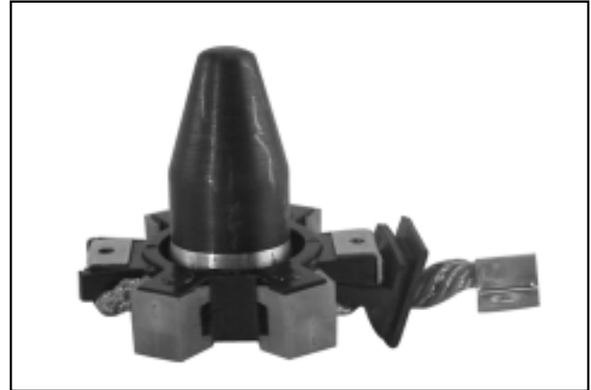
Figure 8-37. Brush Installation Tool with Extension.
