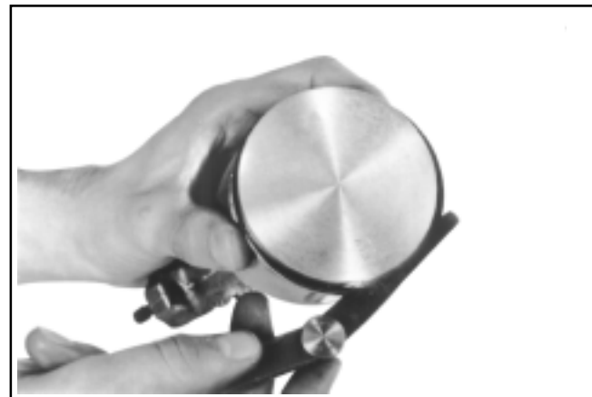
Figure 10-9. Measuring Piston Ring Side Clearance.
