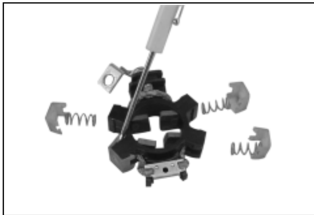
Figure 8-36. Removing Retaining Clips.
