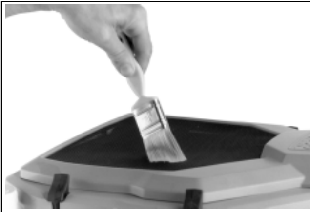
Figure 4-1. Cleaning Air Intake Screen.
