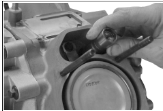
Figure 9-67. Removing Lifters from Lifter Bores.
