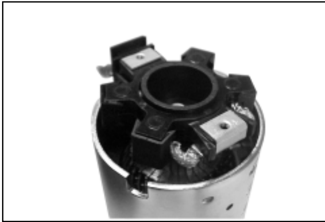
Figure 8-35. Installing Brush Holder Assembly with Supplied Tube.
