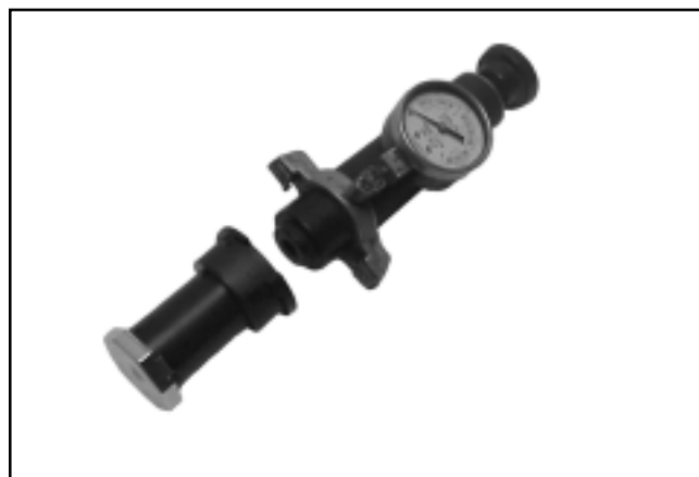
Figure 7-11. A Typical Tester and Adapter.
