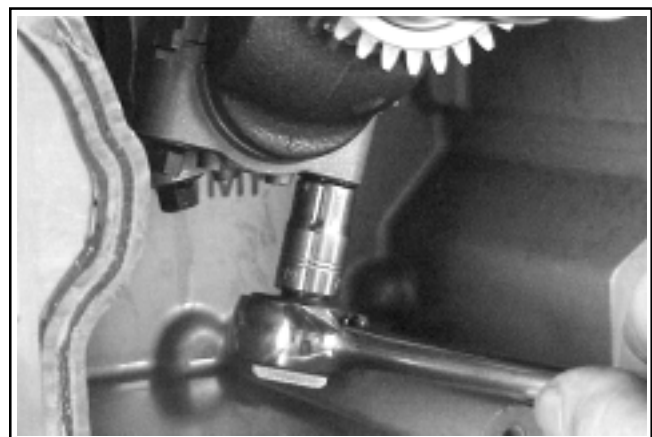
Figure 9-77. Removing Connecting Rod End Cap.
