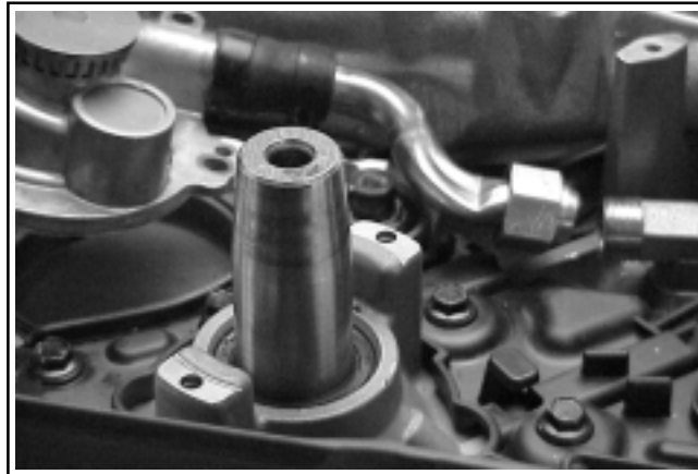
Figure 9-46. Lifting Out Water Pump and Transfer Tube.
