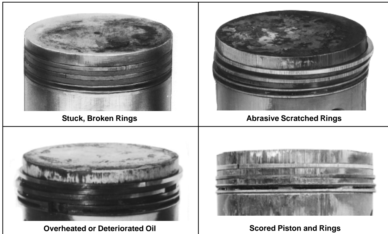
Figure 10-7. Common Types of Piston and Ring Damage.
