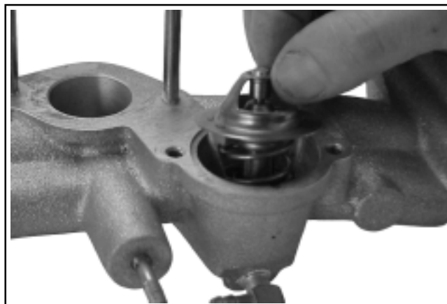
Figure 11-46. Installing Thermostat in Manifold.
