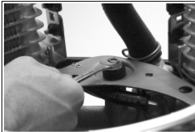
Figure 9-31. Removing Center Mounting Nut.
