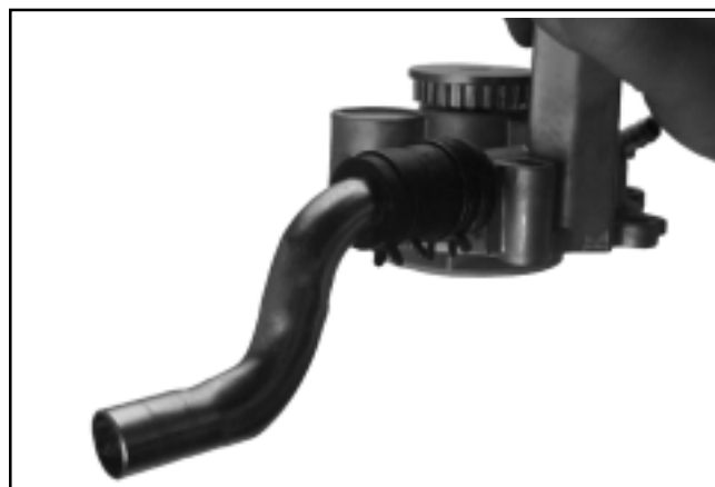
Figure 11-61. Tube and Second Clamp Installed.
