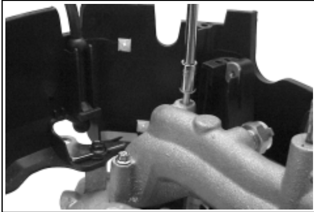
Figure 9-52. Removing Remaining Intake Manifold Screws.
