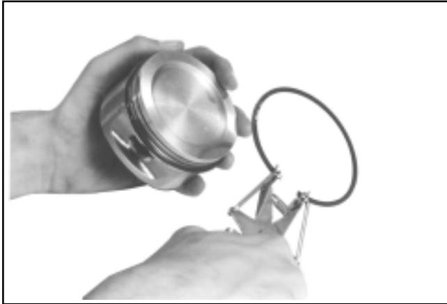
Figure 10-10. Installing Piston Rings With Expander.
