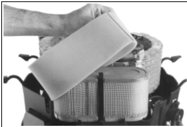
Figure 4-7. Removing Precleaner from Paper Element.
