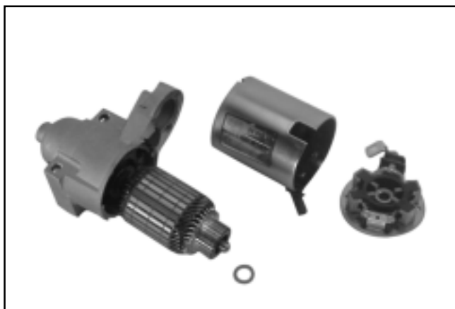
Figure 8-18. Starter Frame Removed.
