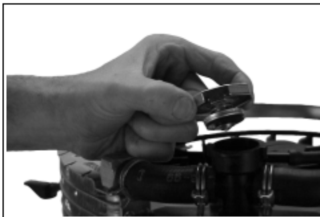
Figure 9-8. Removing Radiator Cap.
