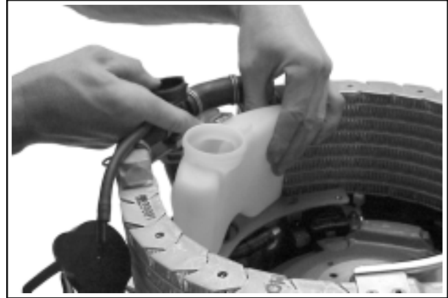
Figure 9-25. Removing the Reservoir.
