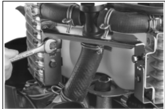
Figure 7-6. Loosening Retainer Bracket Mounting Screws.
