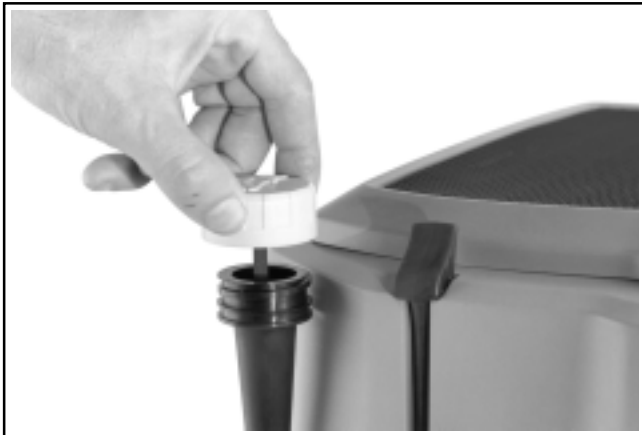
Figure 9-2. Removing Oil Fill Cap/Dipstick.
