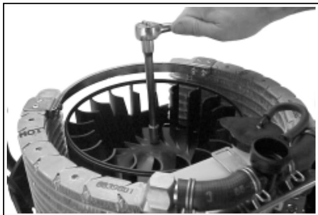
Figure 9-22. Removing Flywheel Fan.
