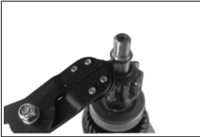
Figure 8-22. Removing Retaining Ring.
