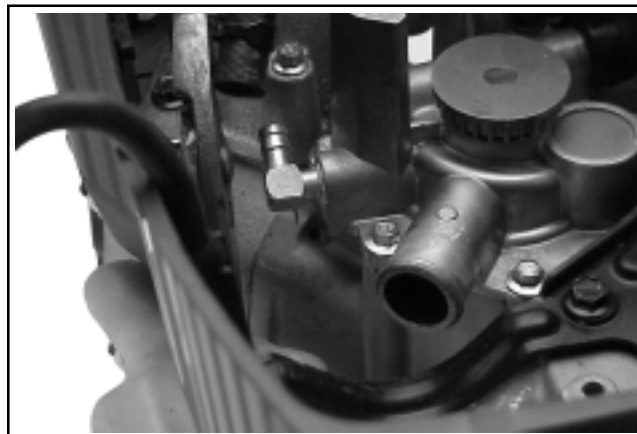
Figure 9-43. Removing By-pass Hose from Water Pump Fitting.
