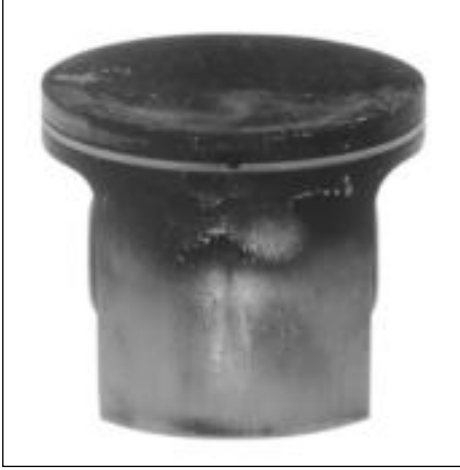
Inlet side. The piston ring is stuck in its groove. Black discolouration under the piston ring due to blow-by.
