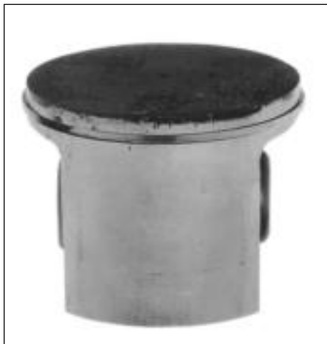
Small score marks and a matt, grey surface on the piston's inlet side caused by fine dust particles.
