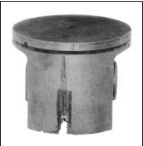
Extensive damage to the piston's inlet side.
