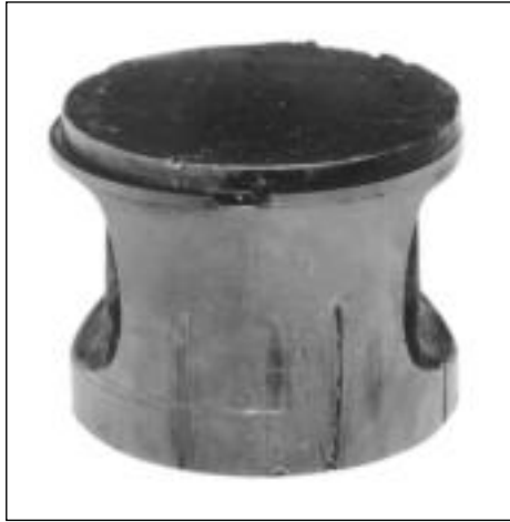
Deep, irregular grooves caused by a loose circlip. Shown here on the piston's inlet side.
