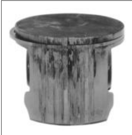
Medium to deep scores along the entire piston skirt on the exhaust side.
