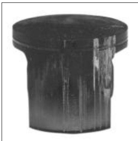
Medium to deep scores on the exhaust side. The piston ring is stuck in the groove. Black miscolouration under the piston ring due to blow-by.
