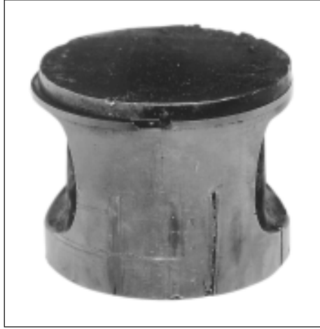
Deep, irregular grooves caused by a loose circlip. Shown here on the piston's inlet side.
