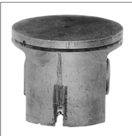
Extensive damage to the piston's inlet side..
