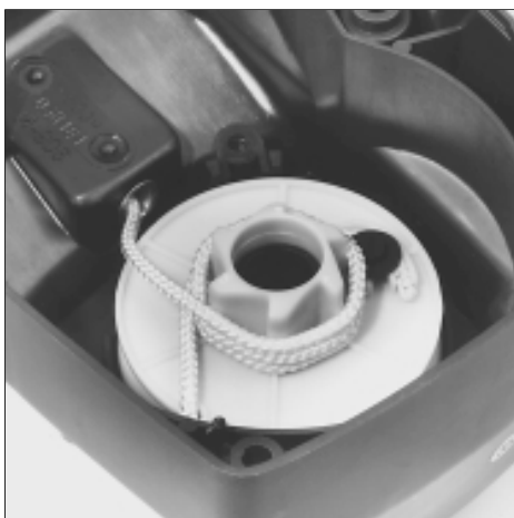
Tension the return spring.
