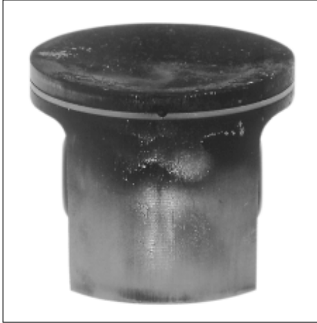
Inlet side. The piston ring is stuck in its groove. Black discoloration under the piston ring due to blow-by.
