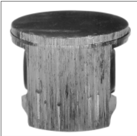
Heavy scoring along the entire piston skirt on the exhaust side.
