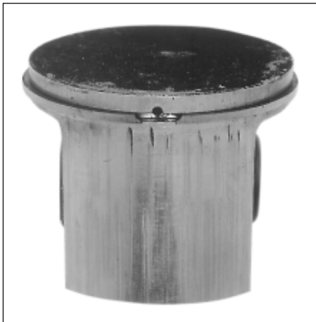
The piston scored and worn from the piston ring down on the inlet side.
