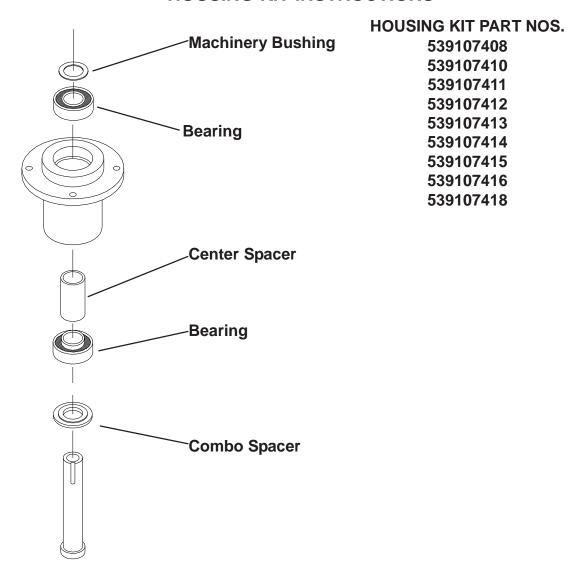
Assemble spindle housing as shown. Make sure to orient the bearings with the extended inner race to the inside of housing.
