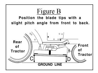
This procedure covers most Husqvarna consumer riding mowers. You may, however, find different style adjustment linkages and deck hangers in use or models where side to side adjustment can only be done on one side. The above guidelines still apply. Please contact your technical service representative for any questions.
