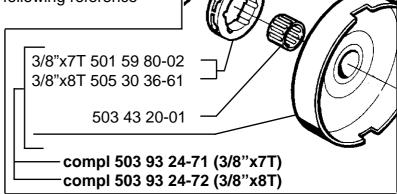
The following variants retain the clutch drum **with** ventilation holes:
