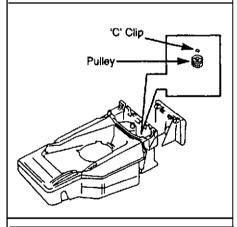
FIT REPLACEMENT PULLEY, ENSURING THAT THE DRIVE PIN IS CORRECTLY LOCATED. RE-ASSEMBLE PARTS IN REVERSE ORDER.
