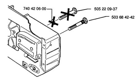
The previous bar bolt, ref. no. 505 22 09-37, can be used in the earlier as well as the later design of crankcase.
