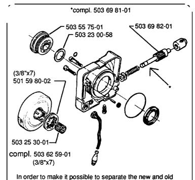
piston, we have marked the new with a turned groove.
