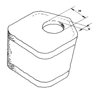
15. The front hand guard of the chain brake has been reinforced and the  $_{\rm material}$  changed. Marking 90-02.
