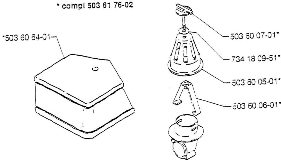
There is also a complete kit available, which includes a cylinder cover, air filter, filter holder and filter oil. Ref. No. 503 61 76-01
