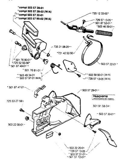
Note that parts with the designation W/A are valid only for the models 266 and 268 equipped with wrap-around handle.
