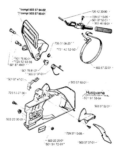
The new chain brake is introduced from serial number 281 -9260401 288-9270400
