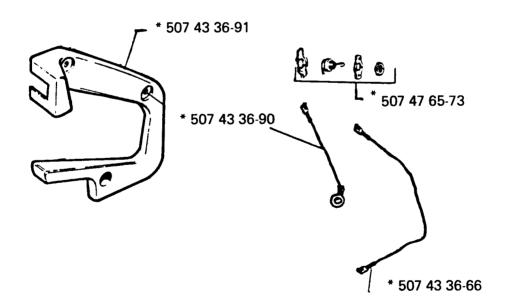
NOTE! For earlier manufactured saws there is a kit available, consisting of stop switch compl. and left handle half. The Ref. No. of the kit is 507 47 65-75.
