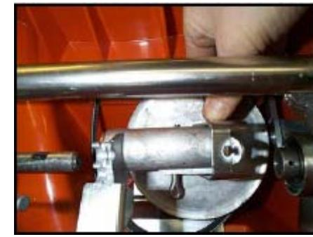
F. Set the shaft, the flat washers and the plastic glide bearing from the top of the variator assembly to the side to be reused. The rubber drive disk and the variator assembly can be discarded.
