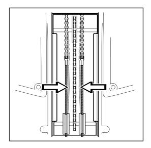
When necessary the wires can be tensioned by tightening the adjusting nuts one on each side of the machine.
