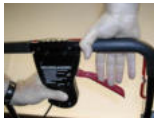
3. Release trigger and push trigger to end of stroke while holding button
