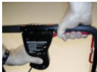
2. Push reset button while holding trigger
