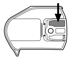
The chain oil is pumped into the chain lubrication hole on the left side of the bar. See figure 3.
