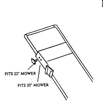
Attach Handle Bracket (C) to Lawnmower handle using wing nut provided on handle bar of mower.
