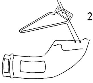
Attach Chute Mounting bracket w/Wire (B) to Plastic Chute (A) using 2 ea. 1/4-20 x 1/2" THMS (H) and 2 ea. 1/4-20 Locknuts (I). Insert 1/4-20 x 1/2" THMS (H) from inside of Plastic Chute (A), up through holes in Plastic Chute (A) and Chute Mounting bracket w/Wire (B). Secure with 1/4-20 Locknuts (I) on top of Chute Mounting Bracket (B). Tighten securely.
