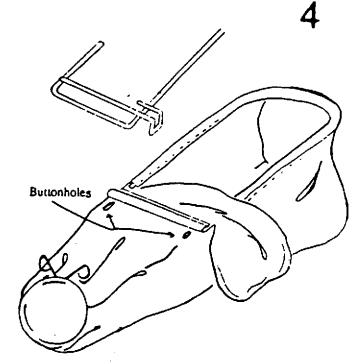
Ends of Bag Frame (D) <u>must</u> be inserted through buttonholes in bag first and then ends of hairpin (sewn in bag) can be pushed on as far as possible. Attach plastic extrusion to first horizontal bar on bag frame (D).
