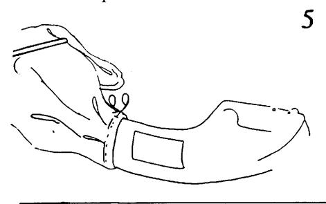
Attach Bag (E) to Plastic Chute (A). Squeeze Clamp Ring (G) and slide bag onto Plastic Chute (A), making sure Bag goes over ridge on Plastic Chute (A). Release Clamp Ring (G), and Bag will fit securely on Plastic Chute (A).
