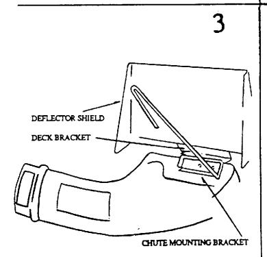
Hook Chute Mounting Bracket w/Wire (B) over deck bracket on lawnmower. When in place, Wire will hold deflector shield up. LEAVE PLASTIC CHUTE (A) ON MOWER DECK.
