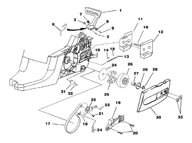
z3350b Chain Saw UT-10759 Clutch - Chain Brake - Drive Case Cover Page 6 of 14
