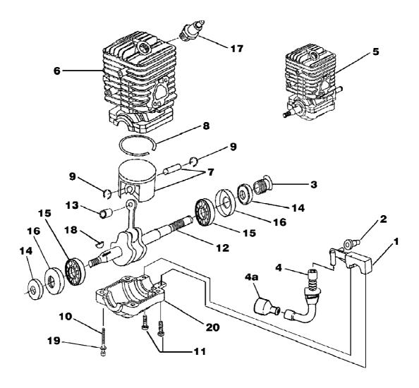
i4550b Chain Saw UT-10834 Engine Internal - Oil Pump Page 10 of 14
