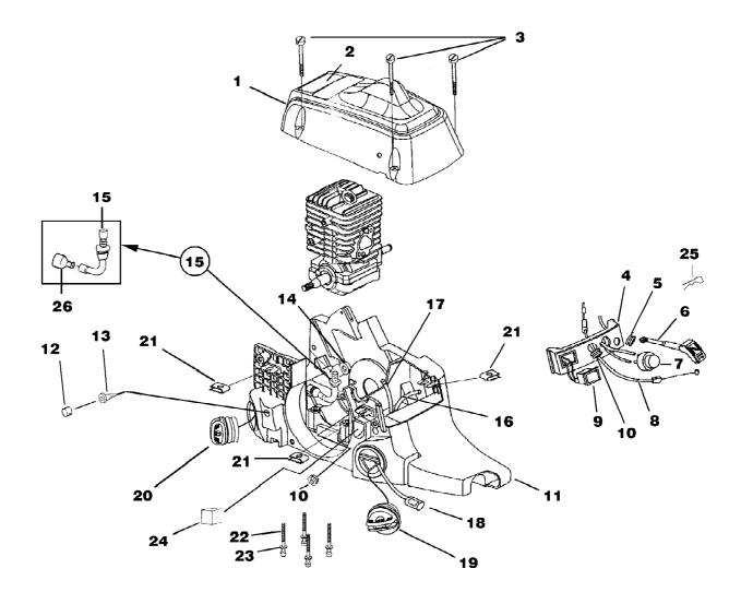
i3850b Chain Saw UT-10758 Engine Housing - Fuel Tank - Oil Tank Page 8 of 14
