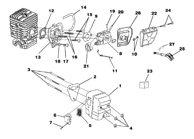
i3850b Chain Saw UT-10758-A Carburetor - Muffler - Air Filter Page 4 of 14
