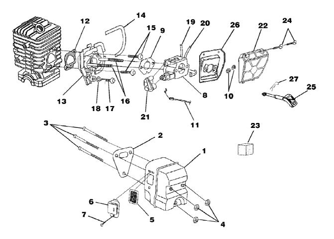
d3850bc Chain Saw UT-10837 Carburetor - Muffler - Air Filter Page 4 of 14
