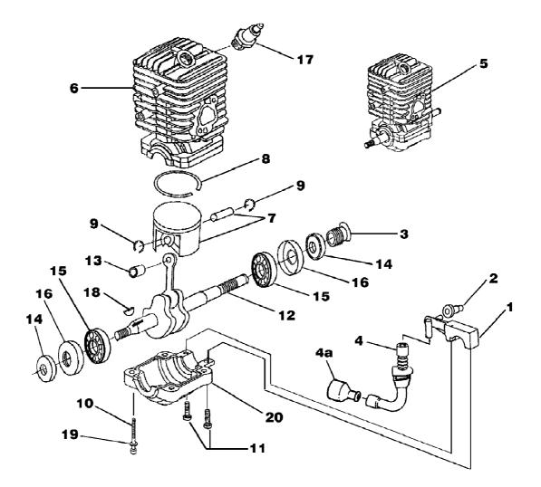
d3850bc Chain Saw UT-10837 Engine Internal - Oil Pump Page 10 of 14
