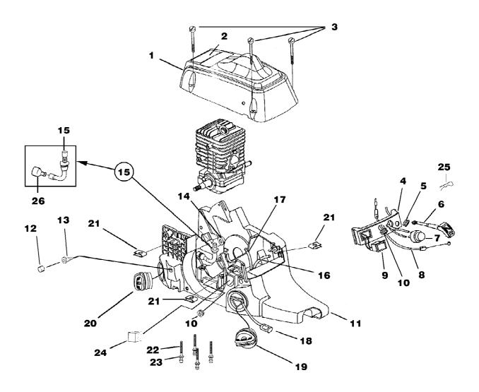
d3850bc Chain Saw UT-10837 Engine Housing - Fuel Tank - Oil Tank Page 8 of 14
