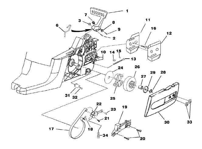
d3850b Chain Saw UT-10833 Clutch - Chain Brake - Drive Case Cover Page 6 of 14
