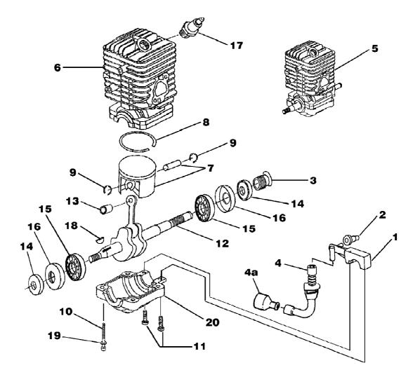
d3850b Chain Saw UT-10833 Engine Internal - Oil Pump Page 10 of 14
