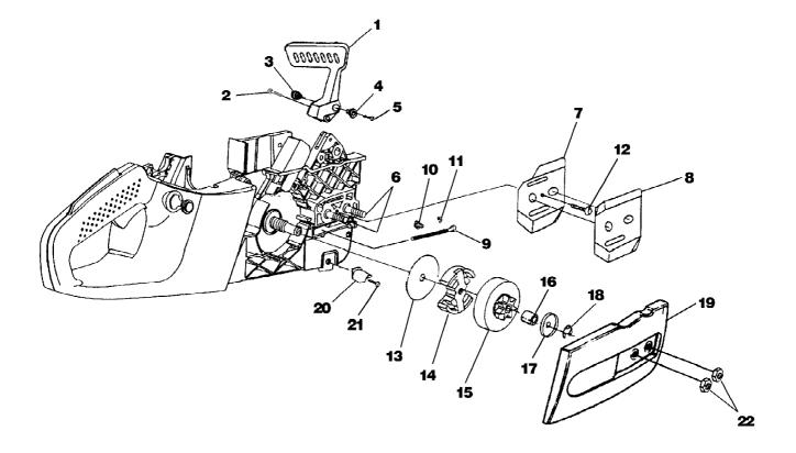
d3800c Chain Saw UT-10783-A Clutch - Hand Guard - Drive Case Cover Page 6 of 14
