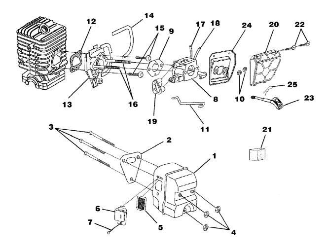
d3800c Chain Saw UT-10783-A Carburetor - Muffler - Air Filter Page 4 of 14
