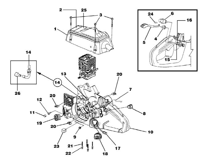
d3800c Chain Saw UT-10783-A Engine Housing - Fuel Tank - Oil Tank Page 8 of 14
