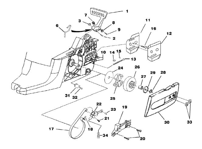
b2316 Chain Saw UT-10936 Clutch - Chain Brake - Drive Case Cover Page 6 of 14
