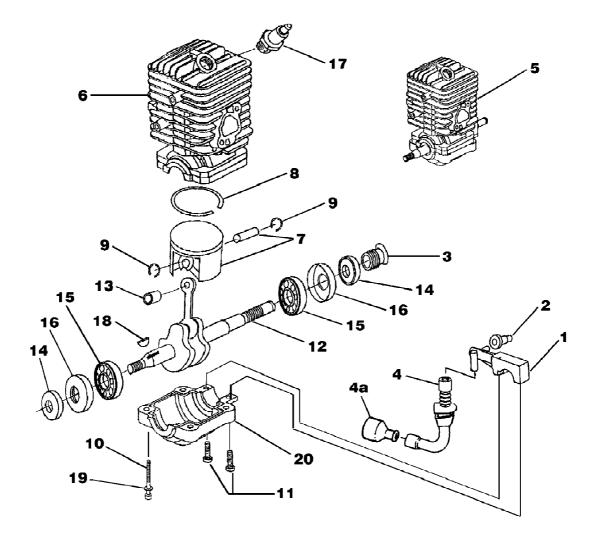
b2316 Chain Saw UT-10936 Engine Internal - Oil Pump Page 10 of 14
