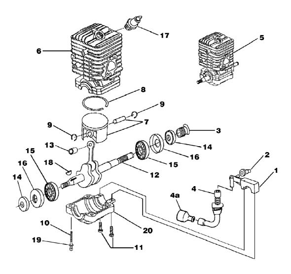
b2014 Chain Saw UT-10934 Engine Internal - Oil Pump Page 10 of 14
