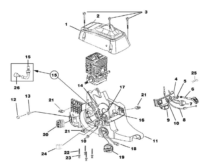
BCS35 Chain Saw UT-10878 Engine Housing - Fuel Tank - Oil Tank Page 8 of 14
