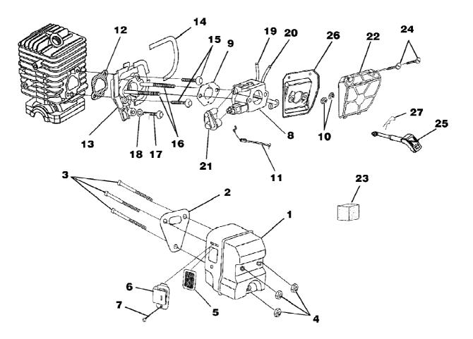
23av w/cc Chain Saw UT-10822 Carburetor - Muffler - Air Filter Page 4 of 14
