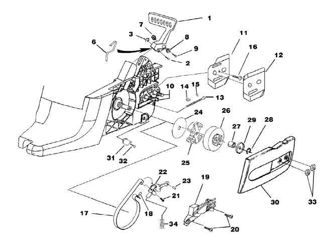
23av w/cc Chain Saw UT-10822 Clutch - Chain Brake - Drive Case Cover Page 6 of 14
