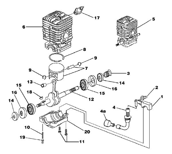
23av w/cc Chain Saw UT-10822 Engine Internal - Oil Pump Page 10 of 14
