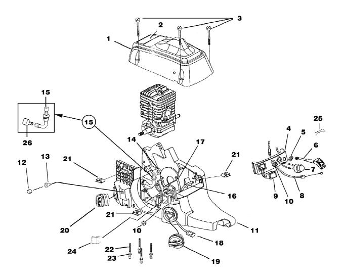
23av w/cc Chain Saw UT-10822 Engine Housing - Fuel Tank - Oil Tank Page 8 of 14
