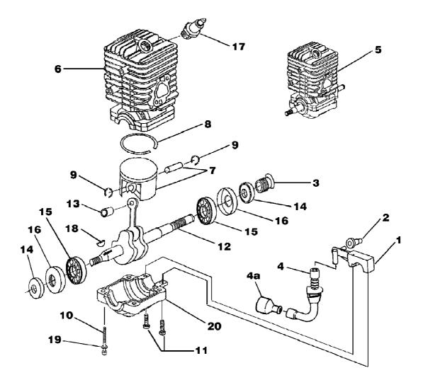
23av Chain Saw UT-10772-A Engine Internal - Oil Pump Page 10 of 14
