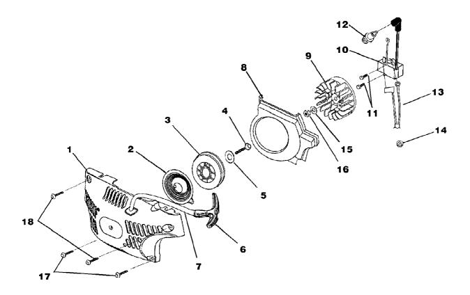
20av w/cc Chain Saw UT-10771-A Starter - Ignition
