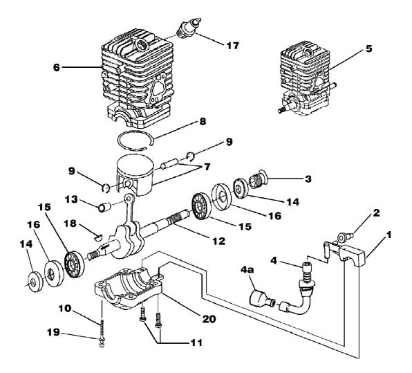
20av w/cc Chain Saw UT-10771-A Engine Internal - Oil Pump Page 10 of 14
