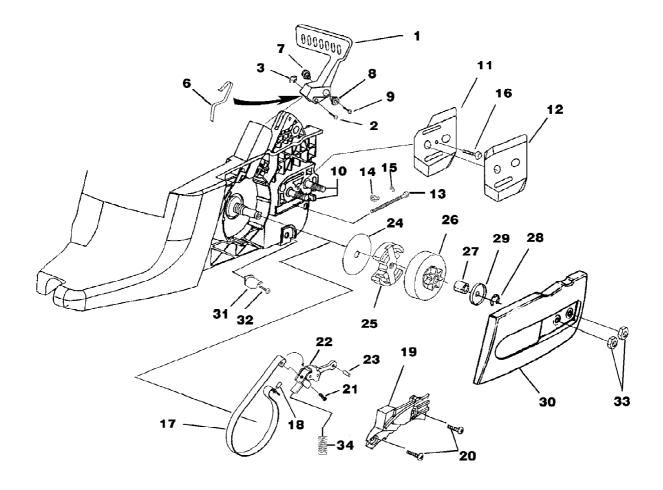
20av w/cc Chain Saw UT-10771-A Clutch - Chain Brake - Drive Case Cover Page 6 of 14
