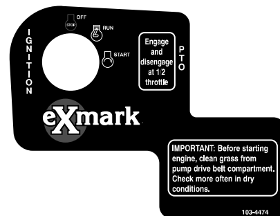
PART NO. 103-4474 LOCATION: Top Front of RH Fuel Tank
