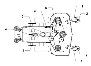
c) Lubricate pivot points with a spray penetrating lubricant as directed below.
