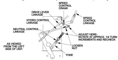
FIGURE 19 HYDRO DRIVE LINKAGE ADJUSTMENT
